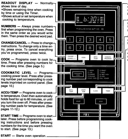
STOP — Stops oven. The oven can also be stopped by opening the door.
