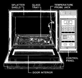
NOTE: DO NOT STORE TEMPERATURE PROBE IN RADARANGE OVEN.
